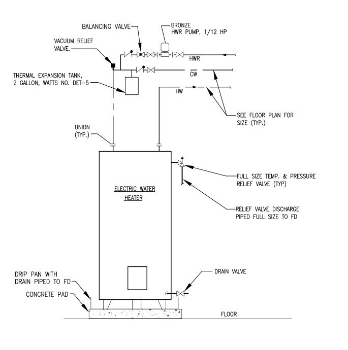
ELECTRIC WATER HEATER (WITH HWRP)
